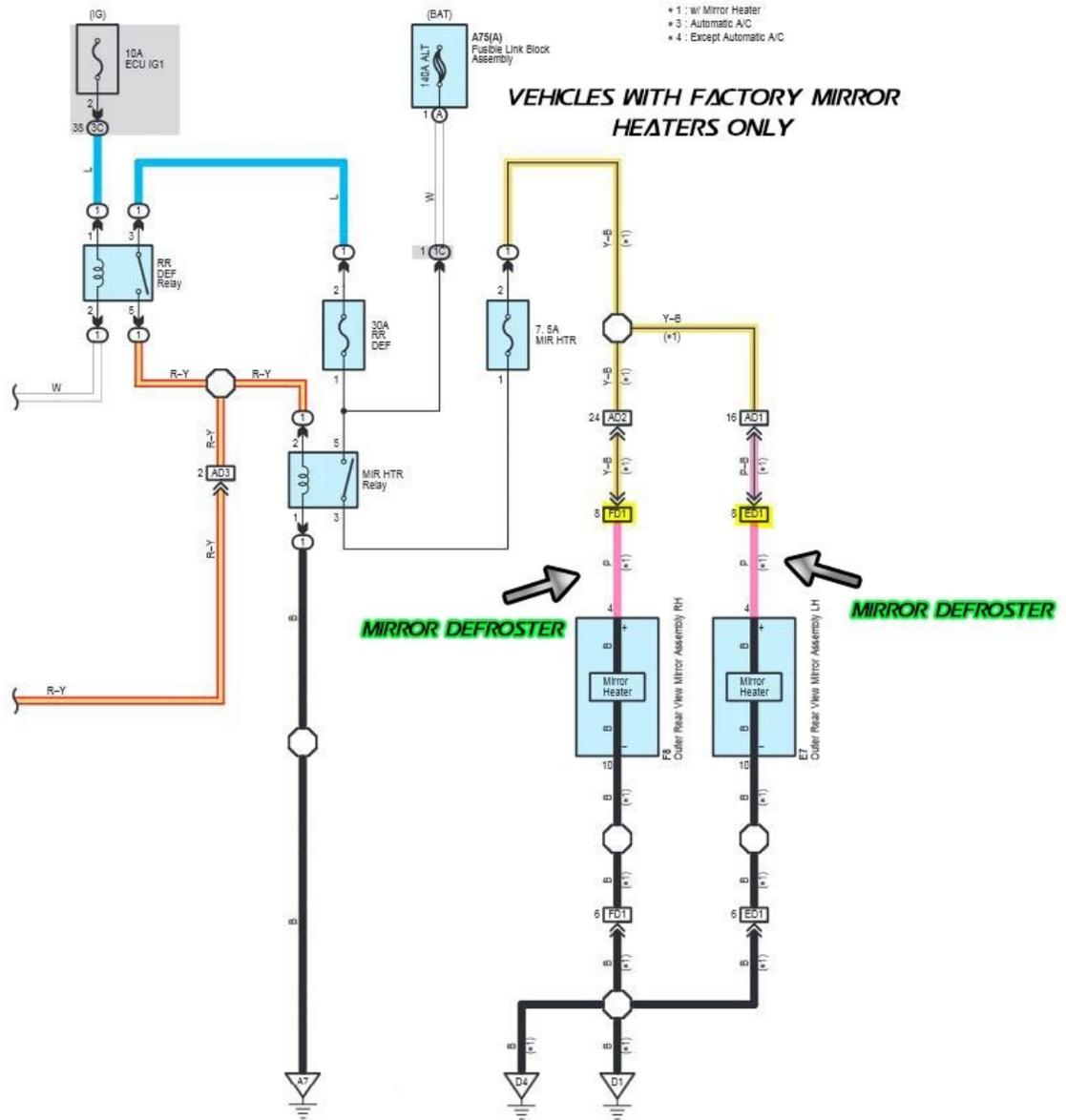
As far as ground points (for the negative), you can find an existing negative wire, use an existing bolt and eyelet grounding end, or tap into the body to ground everything.
