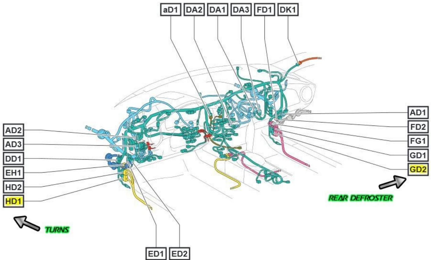
The wires below are located in HD1. This is the plug on the driver's side.
