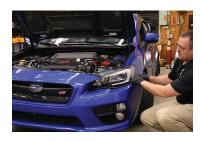
3. With the bolts and rivets removed, detach the bumper from the car by pressing the clips located along the side of the bumper below the headlight. Repeat on the other side. Pull straight back and set the bumper aside on a soft surface.
