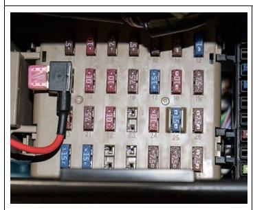
Next locate the fuse box by the driver's side door. It is located around the level of your knee when seated in the driver's seat. Remove the cover.
