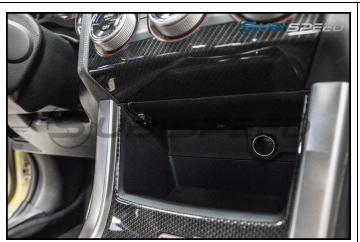
Next, run the wires to the center console or another area and drill a 20mm hole to mount the switch. To gain access behind the AC controls, you can use a screwdriver to pry the panel up from its clips.
