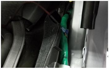
**Test:** The button will work when the ignition is on. Push once to activate and push once more to turn off. If it does not work, please check the add a fuse for burnt / damaged fuses and that the T tap is making proper contact.
