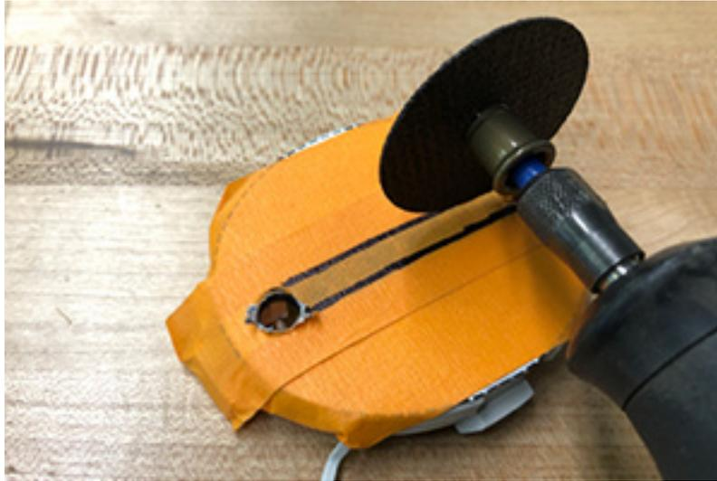
8 Fully cut the inner opening out.
