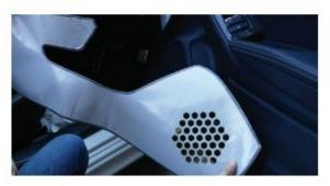
STEP 4: Remove the adhesive backing on the inner portion of the kick guard and carefully place into the mounting location. Remove the backing from the outer edge and remove masking tape. Apply 3M K500 once again on the edges for extra hold.
