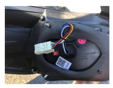
In this picture you can see the wiring bundle was stuck under the gasket which caused an indent and opening for moisture. Be sure to remove the zip tie holding the wiring bundle so it can be clear of the gasket. Depending on model, yours may not have this zip tie.
