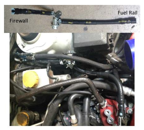
5. Secure the regulator to the bracket that held the plastic line retainer as shown using two 12mm wrenches or a 12mm wrench and socket. You may need to slightly bend the bracket towards the driver's side fender if the regulator is touching the bracket at the bottom of the regulator.
