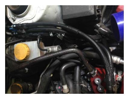
Once installation is completed, reconnect the negative battery terminal and prime the fuel system by cycling the key between the "OFF" and "RUN" positions at 3-second intervals. 4 or 5 cycles will be adequate to re-pressurize the system. CAREFULLY INSPECT FOR LEAKS AND IMMEDIATELY CORRECT IF ANY ARE FOUND!
