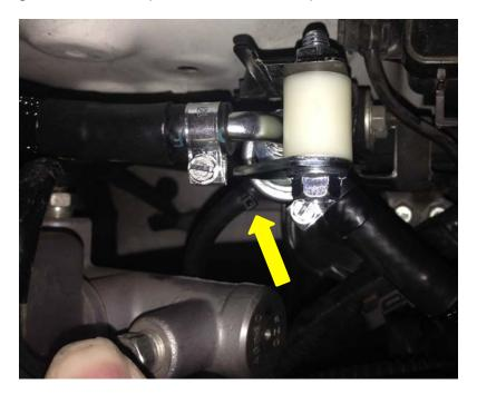
7. Feed Line Orientation – Install the feed line with the sheath covered section going towards the fuel rails.
