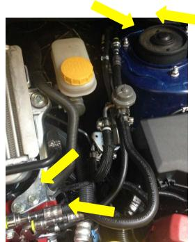
5. Remove the fuel line retainer from the metal bracket using a pair of pliers to pinch the tabs and push it through.
