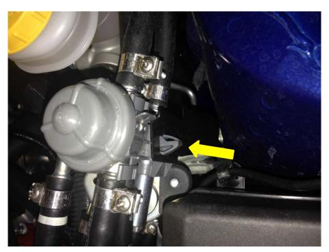
6. Remove the manifold pressure reference from the OEM FPR, and remove the assembly from the engine bay. The factory FPR, dampers and hose assembly is no longer needed. Be careful as excess fuel may continue to drain from the assembly.
