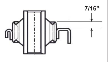
Press the new shell into the control arm until there is 7/16" sticking out on the upper side of the control arm. Install the bushing with p/n 3528 up. Only grease the leading edge to help get the bushing started. Do not grease the I.D. when installing the inner sleeve.
