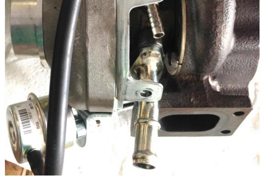
Attach the supplied length of silicone oil drain hose to drain tube and secure with the supplied worm-drive hose clamp.
