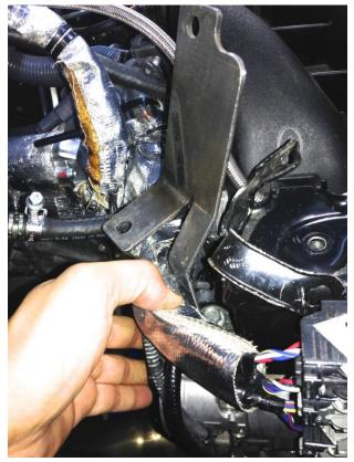
Install the supplied nut and bolt into the bracket's center connection, which mates to a plastic tab on the back of the intake manifold as shown below. Leave this connection loose for now as well.
