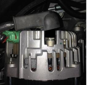
Re-attach the alternator cable to its bracket on the injector cover. It may be necessary to reposition the plastic slide-lock connector on the alternator cable to give additional slack. Ensure there is no contact between the alternator cable and the alternator housing, as this can cause an electrical short. Slide the gray rubber shroud back over the connection.
