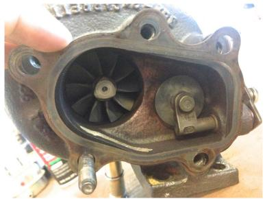
Install downpipe. Apply light coating of anti-seize to the supplied fasteners. Attach downpipe to turbocharger housing using the provided bolts with washers and the single flanged nut. Use the supplied washers under bolt heads. Tighten fasteners in a star pattern to ensure proper gasket sealing. Tightening torque is 25 ft-lbs.
