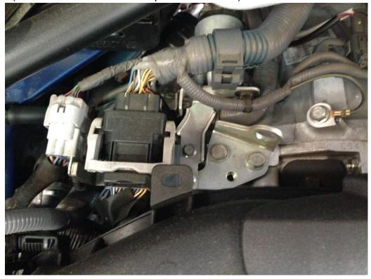
Separate the injector computer from the injector cover by removing the three 10mm-head bolts. Remove the two 12mm-head bolts that fasten the injector cover to the engine block. Release the slide-lock plastic connector holding the alternator cable to the injector cover's front bracket. Remove injector cover.
