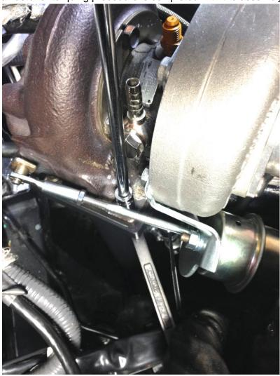
Loosen and remove the two 10mm-head bolts attaching the turbocharger to the bracket. Loosen and remove the two 14mm-head bolts attaching the up pipe to the exhaust manifold. Pull the mated turbo/up pipe assembly out of the car. Tighten the 12mm-head bolt that fastens the bracket to the injector cover. Socket access is tight in this area; we recommend using a 12mm wobble socket. Tighten the 10mm-head bolt/nut connection that fastens the bracket to the intake manifold.
