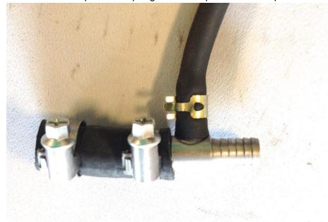
Locate the brake booster connection behind the intake manifold. Disconnect this connection and discard the OEM spring hose clamp.
