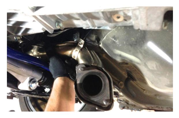
After removing overpipe, lower engine back onto mounts and re-install 14mm-head nuts in subframe. Torque nuts to 33 foot-pounds. Ensure alignment dowels properly enter slots when lowering engine back down.
