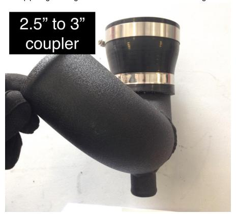
Leave all hose clamps loose until final tubing orientation is achieved. Install angled upipe onto throttle body in the orientation shown below.
