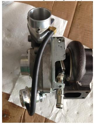
Install the oil drain tube onto the turbo's oil drain flange using the supplied gasket and fasteners. Orient the oil drain tube so that it curves towards the aluminum compressor
