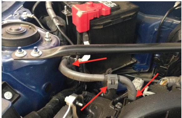
Remove the two 14mm-head bolts holding down the gold wiring harness bracket. Release the wiring harness connections attached to it and remove the bracket from vehicle. **Optional:** Remove bracket and cut leaving engine hoist eyelet and 3 closest holes (2 14mm-head bolt holes and open threaded hole). Reinstall to retain bracket.
