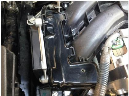
Using a vice or channel locks, bend the two rear bracket tabs forward until they are nearly flush with the top surface of the injector cover - this will make room for the turbocharger. You may remove these two tabs entirely with a cutoff wheel if desired.
