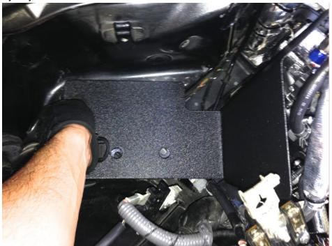
Reinstall the plastic battery tray, ensuring bump alignment in the holes. Place battery back in tray, ensuring that tray and heatshield stay aligned. Once battery has been placed in tray, slide battery as far towards the fender/a-pillar as the tray will allow – moving the battery away from the turbo helps keep it cool. Reinstall battery tie-down tray and associated hardware. Reconnect battery leads.
