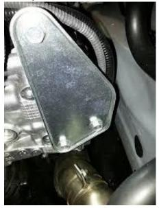
Remove the three bolts and gently pry the cam plate off the block. It is factory-sealed to the block with silicone sealant, so it may require some effort to remove. Exercise caution when removing the plate and be careful not to mar the engine block's aluminum sealing surface upon removal. Once the cam plate is removed, clean all silicone sealant from the engine block, again taking care not to scratch or gouge the sealing surface.
