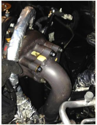
Underneath car, fasten downpipe outlet to front pipe using the supplied fasteners and gasket.
