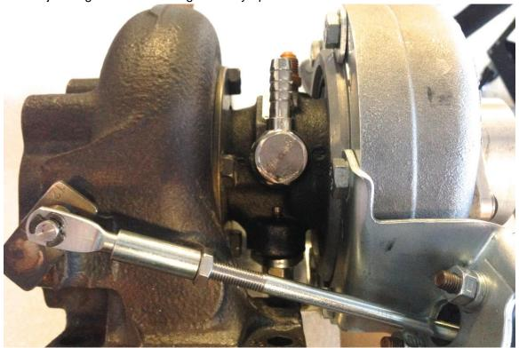
Install the second banjo coolant fitting, again ensuring use of a crush washer on either side of the banjo fitting. Orient this fitting as shown below: roughly 15 degrees right of vertical-down.
