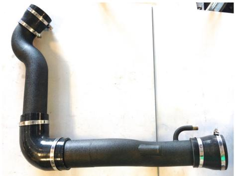
Install tubing assembly between turbocharger inlet and airbox. It may be necessary to adjust pipe protrusion into the silicone connectors during installation. Ensure proper clearance around all piping before tightening hose clamps.
