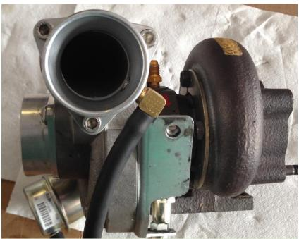
Run the supplied vacuum tubing from the brass fitting on the compressor outlet to the wastegate, routing as shown. Secure using the spring clamps provided.
