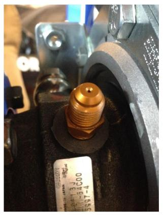
Install the first banjo coolant fitting. Be sure to include a crush washer on either side of the banjo fitting. Orient this fitting vertically up as shown below.
