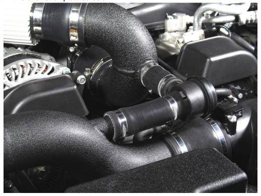
Slide the short length of rubber tubing onto one end of the stainless T-fitting and secure with provided hose clamp. Slide the long length of vacuum hose onto the T's smallest fitting and secure with the provided spring hose clamp. Refer to the picture below.
