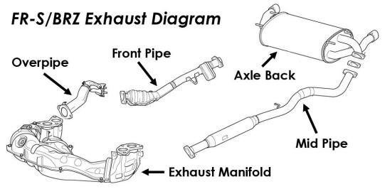
**WARNING:** Exhaust hardware is prone to seizing, even on fair-climate cars. It is recommended to use penetrating fluid and a box-end wrench to avoid damaging fasteners.
