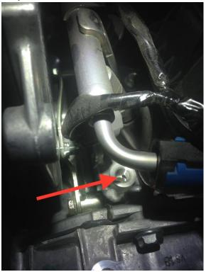
Locate the supplied oil fitting adaptor, and install it into the same hole, using the supplied new crush washer. Tighten this connection until snug. Locate the supplied stainless-braided oil line, thread the end with the straight fitting onto the adapter, and tighten. Reinstall the injector cover, routing the oil line out the rear as shown below. Reinstall the three 10mm-head bolts holding on the injector computer, and the **front** 12mm-head bolt. Leave the rear 12mm-head bolt out at this time.
