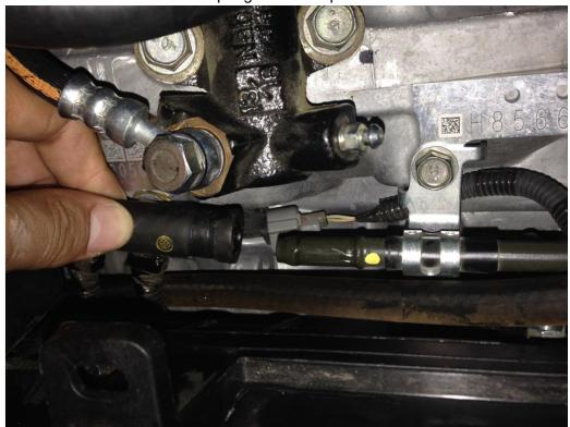
Slide the T-fitting into place and secure on both ends using the supplied worm-drive hose clamps.
