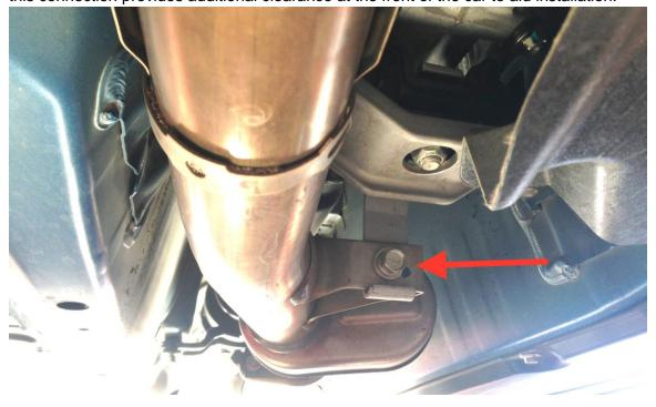
Remove overpipe. The overpipe is often difficult to remove due to space constraints. To gain additional clearance, remove the two 14mm-head engine mount nuts inside the front subframe pockets shown below.
