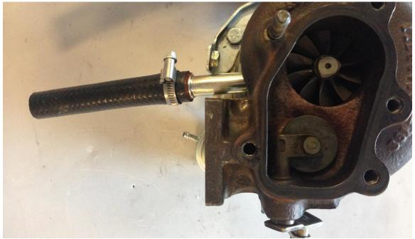
Install the gold oil fitting into the top of the turbocharger oil supply port and tighten until
