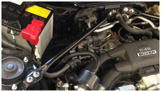
Remove noise generator and intake tube. The noise generator is secured by two 10mm-head bolts on top of the injector cover, two push-lock plastic connectors, and by a pull-to-remove grommet connection in a pocket below the firewall. Remove the intake tube by loosening the two large hose clamps on either end as well as the PCV connection, held by a spring-loaded clamp.
