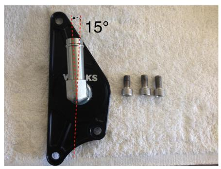
Apply a light film of engine oil to the large rubber o-ring and install it onto the backside of the plate. Install the new cam plate onto the engine using the supplied hardware. Tightening torque is 15 ft-lbs.
