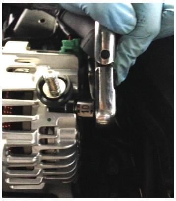
Slide the provided 6mm split lockwasher onto the stud that protrudes horizontally out of the rear of the alternator body. Thread on the provided alternator stud extension piece and tighten. Slip the provided piece of rubber tubing over the alternator stud extender. Re-attach the alternator contact tab and fasten using the original nut and lockwasher.
