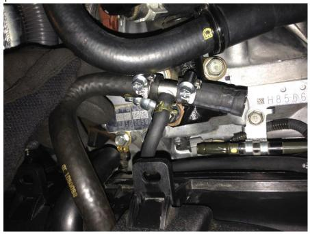
Route the small-diameter vacuum hose up towards the diverter valve. When routing, ensure that the line is not pinched or kinked, and that it is secured and out of the way of moving engine components. Attach the free end of the vacuum hose to the small fitting on the diverter valve, securing with the provided spring clamp.
