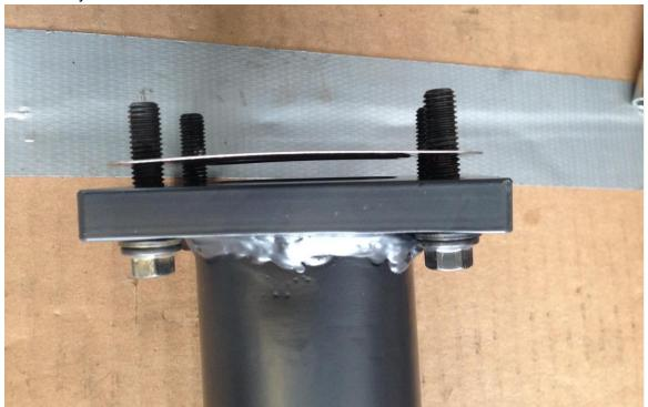
Use the provided black bolts. Install with washers under the bolt heads. Orient the bolts upside down as shown below. Again, ensure that this connection remains loose at this time.
