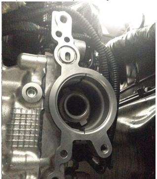
Thread the fitting into cam plate and orient as pictured - the barbed tube should point approximately 15 degrees left of vertical. Tighten the jamnut. Do not overtorque; this fitting only needs to be snug.
