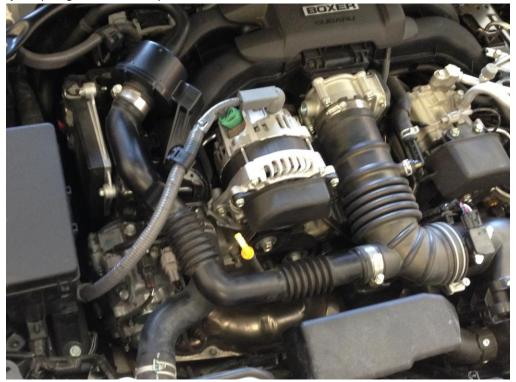
Separate the three tie-down points for the grey battery cable: one push-lock connector on the shock tower, one slide-lock connector on the injector cover bracket, and one push-lock connector behind the intake manifold.
