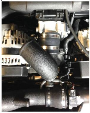
The 1" tube fitting should point straight towards the front of the car as shown. Install finned tube between u-pipe and turbocharger compressor outlet. Clearance between alternator and finned tube can be adjusted by rotating angled u-pipe slightly. Adjust until there is roughly ½" inch clearance between top of alternator and finned tube.
