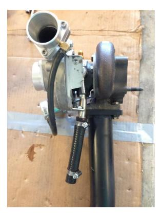
Re-install assembly in car. Remember to install the supplied gasket on the exhaust manifold outlet. Slip the turbocharger's silicone oil drain tube onto the barbed oil fitting and secure with included worm-drive hose clamp.
