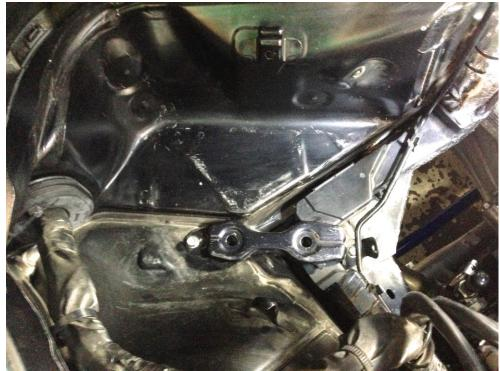
Slide in the provided WORKS heatshield. The two holes in the bottom of the heatshield should align with the two holes in the frame that mate to the bumps on the underside of the battery tray.
