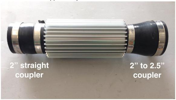
Pre-assemble the angled u-pipe as shown. The larger silicone transition should be installed on the pipe leg that aligns with the smaller diverter valve fitting.
