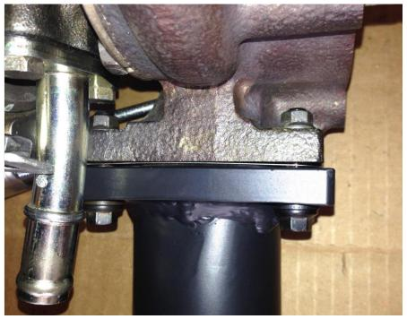
Lower the joined up pipe/turbo assembly into car and test fit. Install and loosely thread the following fasteners:
