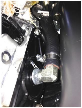
Re-install and tighten the two M6 bolts that fasten the turbo to the bracket.
