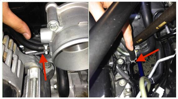
Release the spring clamp on either end of this hose and remove the hose entirely. Because this hose runs underneath the intake manifold, it may require some manipulating to remove.
