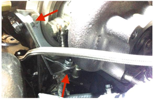
Re-install and torque the two 14mm-head nuts on the exhaust manifold. Again, inspect this junction carefully as an exhaust leak at this location will be time consuming to fix.
