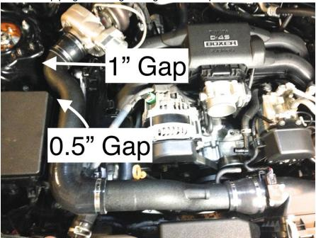
**WARNING:** Avoid excessive tightening torque when installing worm-drive hose clamps. High tightening torque is not necessary to achieve proper sealing. Recommended tightening torque for supplied 9mm-wide worm-drive hose clamps is 29 **inch**-pounds. Over-tightening can damage silicone connectors and crush tubing.
