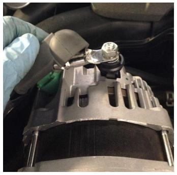
Remove and save the nut and lockwasher that fasten the alternator cable. Remove the circular cap on the backside of the black plastic alternator tab, and then remove the nut underneath it using a 10mm socket. Remove the black plastic connector assembly from alternator.
