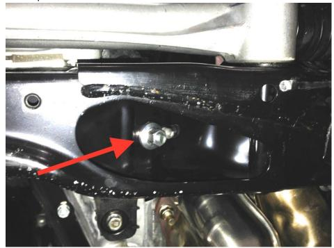
Using a screw jack or floor jack, gently raise the engine/transmission out of the chassis about 1". Use the transmission bellhousing as a jacking point as shown below. Do not to put excessive pressure on the jack point; 1" of lift provides enough additional clearance to easily remove the overpipe.
