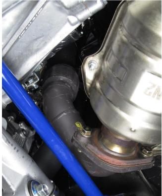
Re-install the 14mm-head bolt that fastens the front pipe to the chassis and remove any straps or support provisions installed to support hanging exhaust. Check around downpipe path for clearance. It may be necessary to rotate or adjust manual transmission grounding wire to move away from downpipe path.
