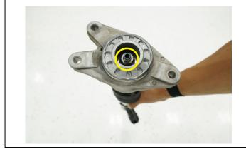
24 INSTALL FACTIONFAB REAR BUMP STOP INTO THE FACTIONFAB REAR DUST BOOT
