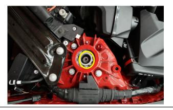
MOVING TO THE REAR, REMOVE THE AERO SHIELD HELD ON BY 4 10mm NUTS
