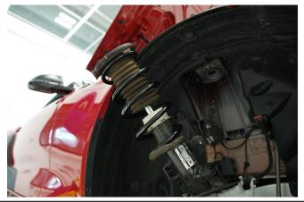
LOWER JACK AND ROTATE ASSEMBLY OUTSIDE OF THE WHEEL WELL, THEN REMOVE SPRING
