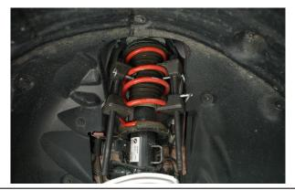
7 REMOVE TOP SHOCK NUT WITH 6mm HEX KEY AND 18mm PASS THROUGH SOCKET
