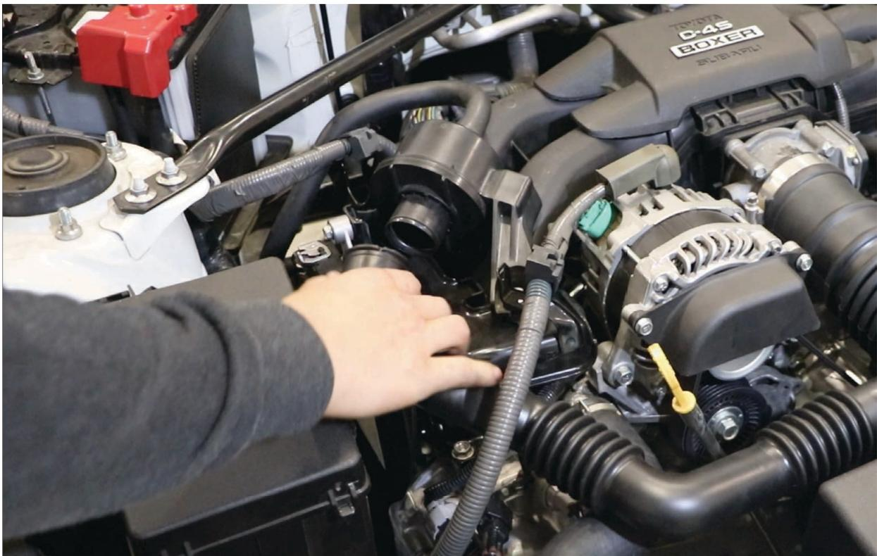
d. Locate and disconnect 4 plugs from the Injector Control Unit, pictured below. Each plug has a unique way to release.
