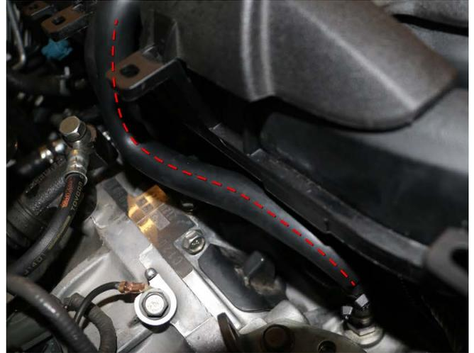
16. Using a 10mm socket or wrench, replace the silver bracket on top of the Driver's LH side of the intake manifold. Refer to Step 6.
