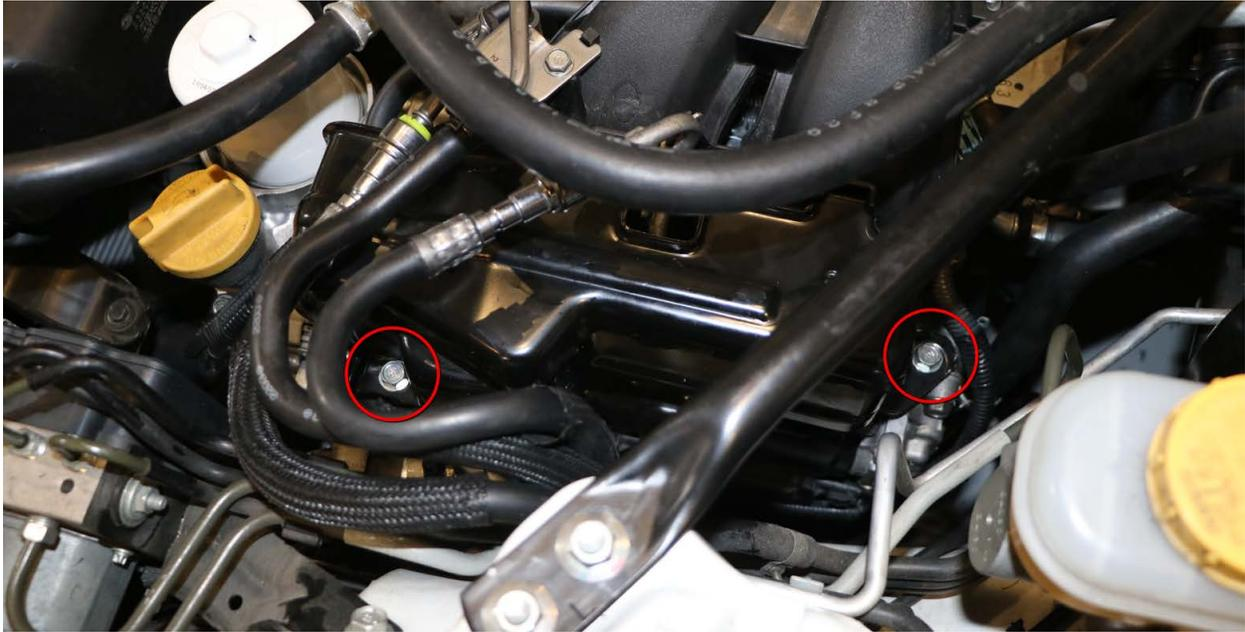
3. Remove Driver's RH fuel rail crash guard/injector control unit, located on the US passenger side of the intake manifold.
