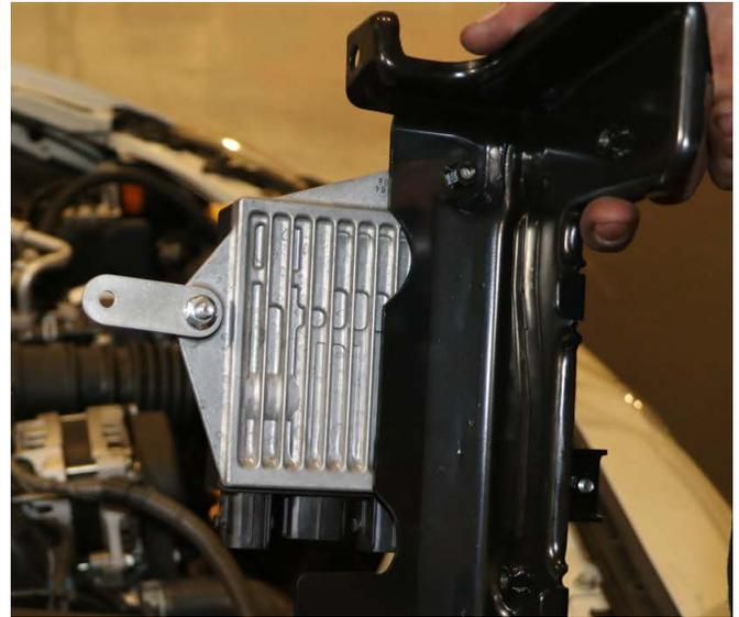
**\*\*VERY IMPORTANT:** This bracket MUST be installed in order to ground the Injector Control Unit. Without it, your vehicle will not be operational.
