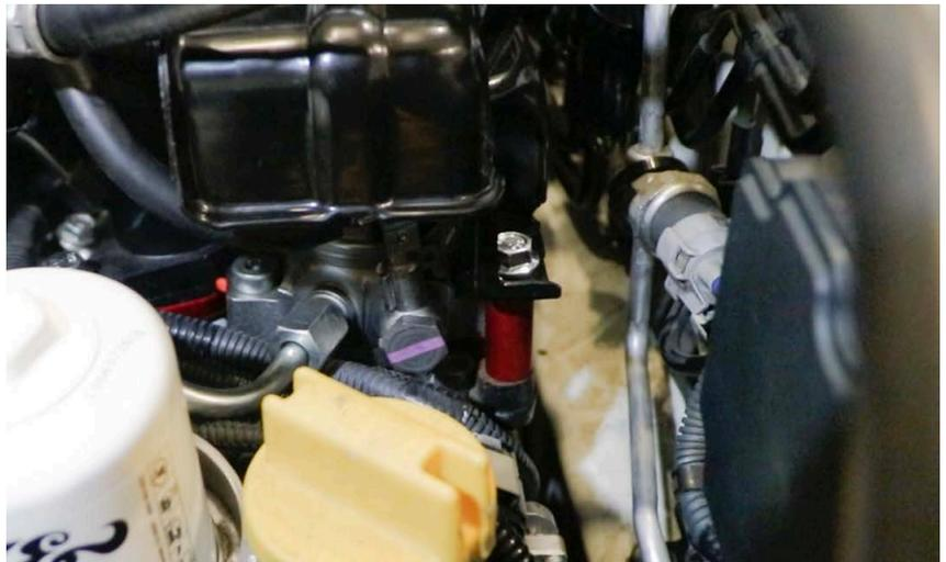
15. Locate the PCV hoses going in to the top of the intake manifold from behind it, close to the firewall. When the Intake manifold was lifted, the PCV hose going in to the top of the intake manifold from the top of the block most likely disconnected from the block. Insert the supplied straight fitting on the open end, and attach the supplied hose extension to the other end. Zip tie both ends to secure the hoses to the straight fitting, and reattach the PCV hose to the block.
