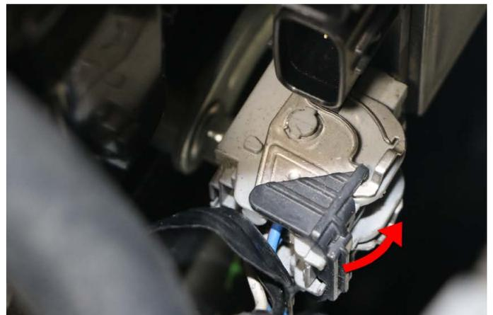
e. Using a 12mm socket with extension, remove the 2 crash guard/injector control unit mounting bolts on top, and using a 10mm socket remove the bottom (3rd) bolt. This bottom bolt will be the only bolt reused, and we recommend storing the other 2 in case you need to later revert your vehicle back to stock.
