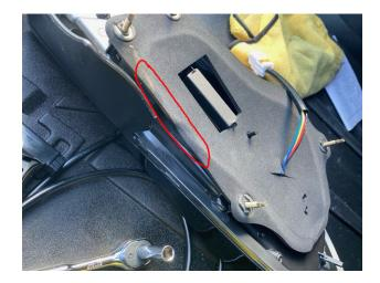
Image shows the edge of the sealing surface covered by the gasket. Ensure the gasket is not creased or pinched anywhere along the sealing surface edge.
