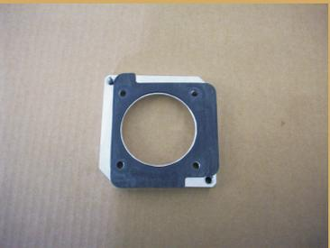
**16** Bolt the throttle body adaptor to the intake manifold. Place the factory gasket between the adaptor and the manifold.
