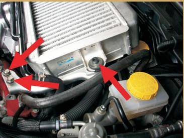
**24** Install the vacuum line and the blow-off valve.
