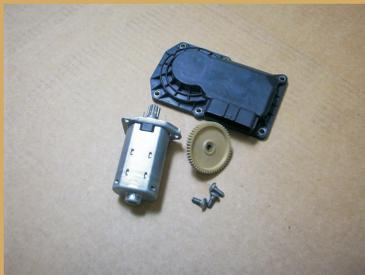
**14** Reinstall the servo motor and the spur gear. Install the throttle body cover.
