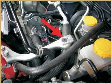
**21** Install the intercooler. Tighten the input and output hose clamps. Install the MAP sensor.
