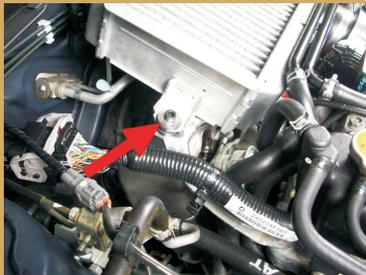
**23** Bolt on the right intercooler mount. Tighten the right intercooler bracket.
