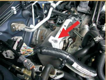
**20** Install the intercooler mount to the right intercooler bracket.
