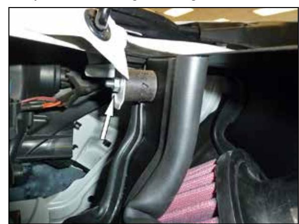
18. Using the factory nut, secure the rubber mounted stud to the core support.
