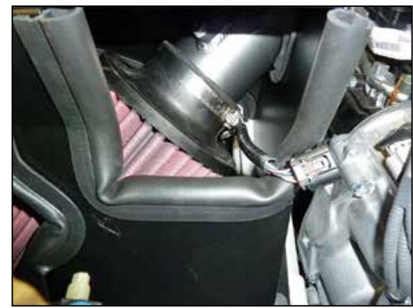
19. Reaching in through the fresh air opening in the heat shield, retrieve the mass air sensor wiring pigtail laying on the frame and connect it to the mass air sensor. Check to make sure that the wire is not pinched or bound with could cause damage to the wiring.
