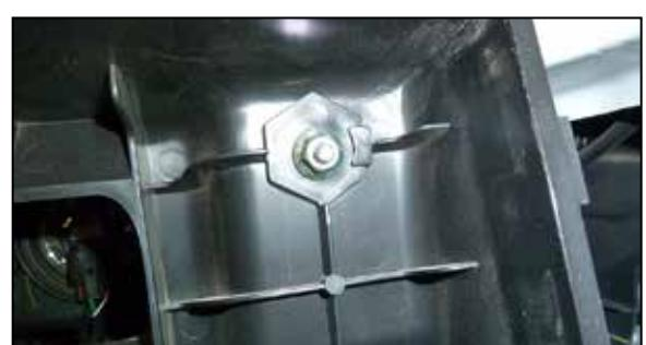
6. Release the air filter housing clips and remove the housing half and factory air filter. Remove the air filter housing retaining nut.
