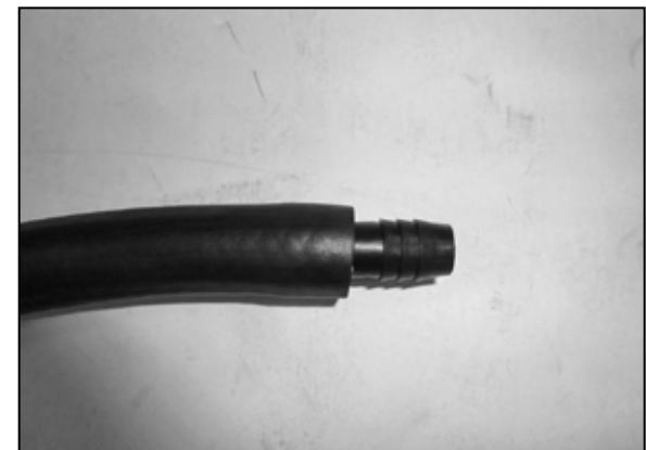
21. Install the provided hose union into the provided crank case vent hose as shown.
