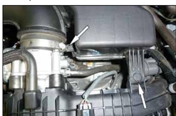
4. Remove the clip that secures the intake plenum to the manifold and then loosen the hose clamp that secures the intake tube to the throttle body.
