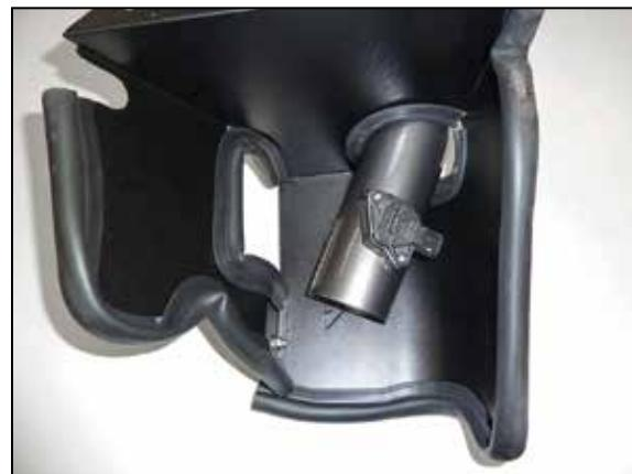
12. Install the AEM® intake tube trough the heat shield, then remove the mass air sensor from the factory housing and install it into the AEM® intake tube using the provided hardware.
