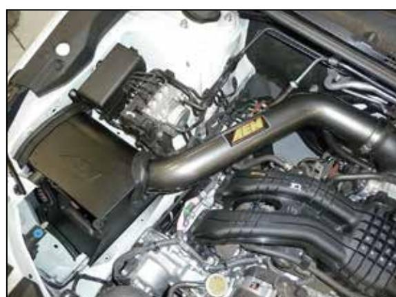
16. Install the intake assembly so the intake tube goes into the coupler at the throttle body and the heat shield rests on the frame and the mounting holes line up correctly.
