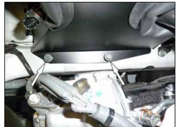
17. Secure the heat shield to the frame with the factory air filter housing mounting bolts.
