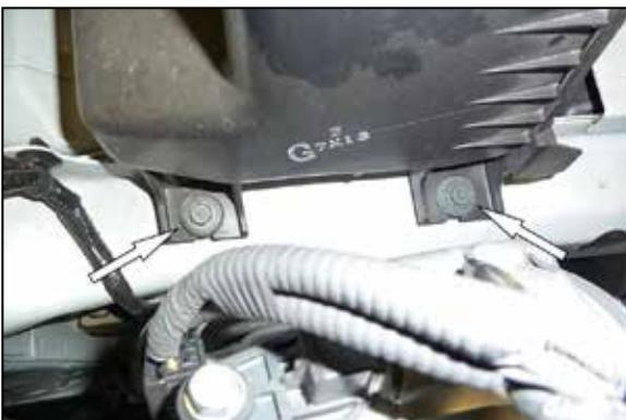
7. Remove the two bolts that secure the air filter housing to the frame rail, then remove the air filter housing.
