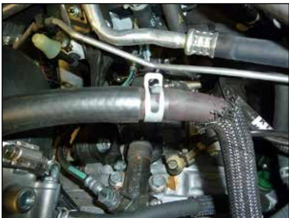
22. Install the crank case vent hose assembly into the factory crank case vent hose and secure with the factory spring clamp.
