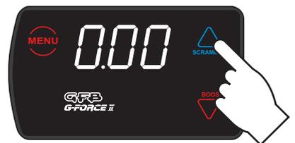
If you want to activate scramble using a remote-mounted button, switch ECU output etc, you need to first connect the blue remote wire to the button/switch/ECU output you want to use (see page 3 for wiring diagram), then set the input to “SCr” (see page 12, “Input Setup”). Once you have done this, the remote input will replicate the function of the up/scramble button, and the up/scramble button will also change colour in the same way to indicate when scramble is active.
