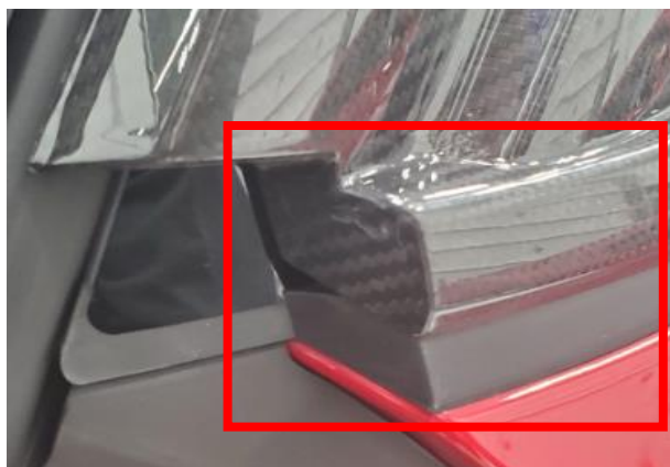
Incorrect: Notice large gap between carbon and trim
