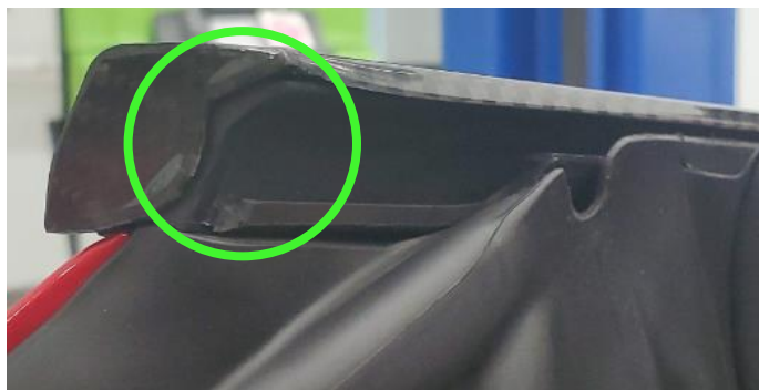
Correct: Notice carbon and door edge are flush
