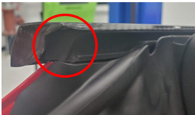
Incorrect: Notice large gap between carbon and door
