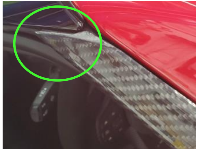
Figure 2: Aligning part ③ with A-pillar
