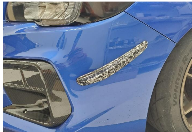
Figure 2: Suggested installation location: 18-21 front bumper
