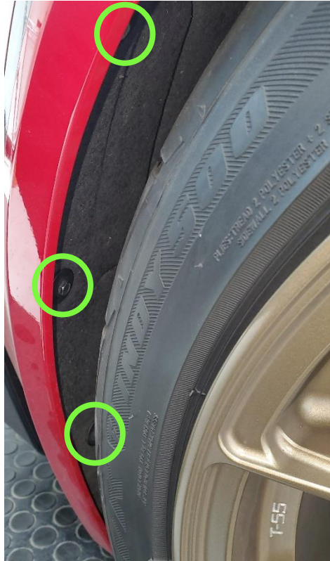
Rear wheel well liner bolt locations (3)
