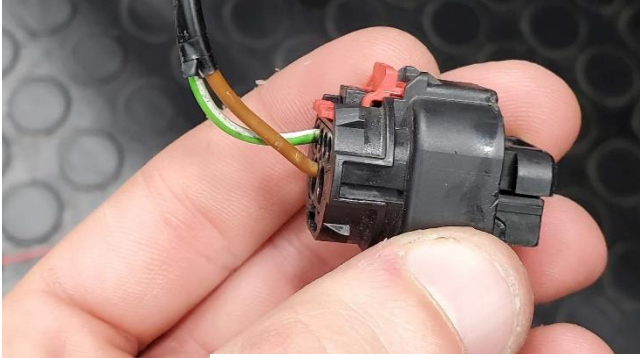
4 th brake light connector with red tab in unlocked position
