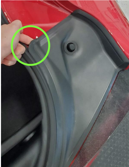
Installed cover, showing pry point
