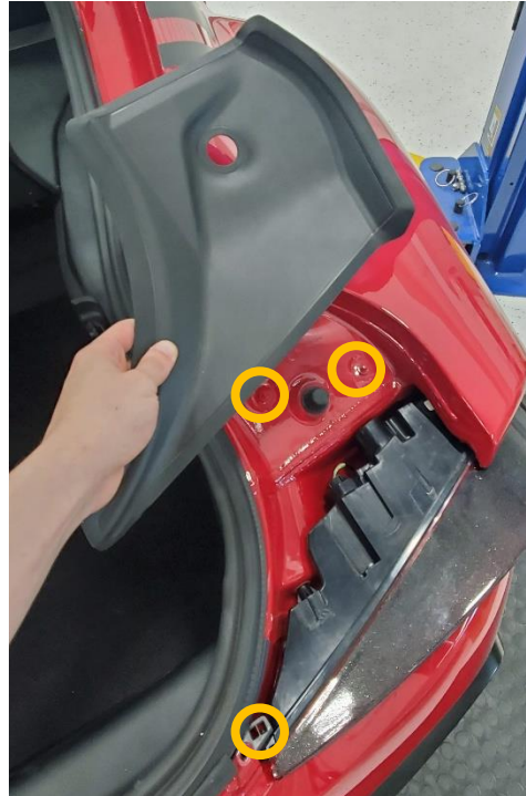
Removed cover, showing clip locations
