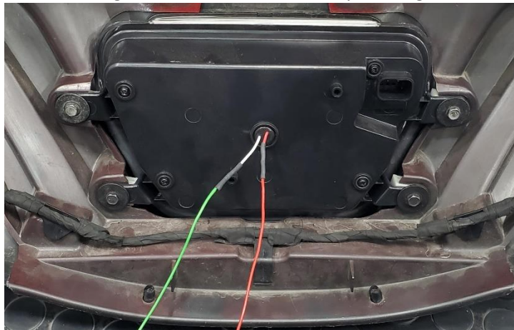
OLM 4 th brake light installed into bumper
