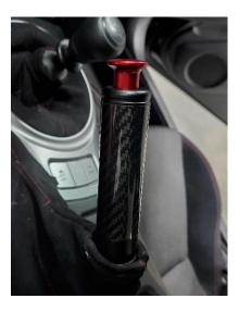
10 – Screw on the button all the way down until it stops. Reverse approximately 2 ½ turns to ensure the button functions correctly.
