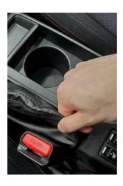
3 – Next, put your hand between the lower seat cushion and the center console and find the bottom of the e-brake boot and plastic trim ring. Pull straight up to release the rest of the clips. The e-brake boot should now be free from the center console.
